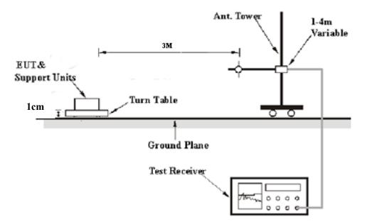
The radiated emission tests were performed in the 3-meter chamber a test site, using the setup accordance with the ANSI C63.10. The specification used was the FCC Part Subpart C limits.
