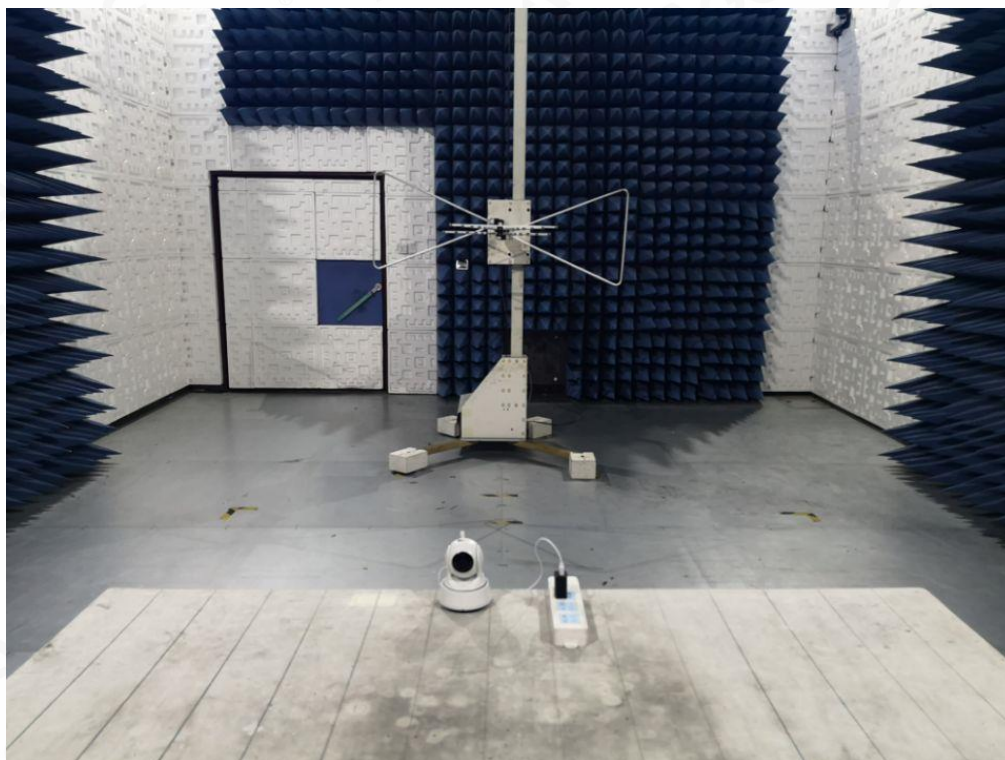
FCC RADIATED EMISSION TEST SETUP ABOVE 1GHZ
