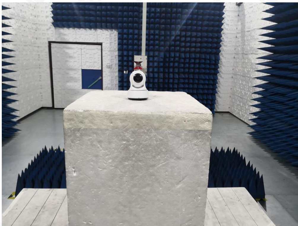
FCC RADIATED EMISSION TEST SETUP ABOVE 1GHZ
