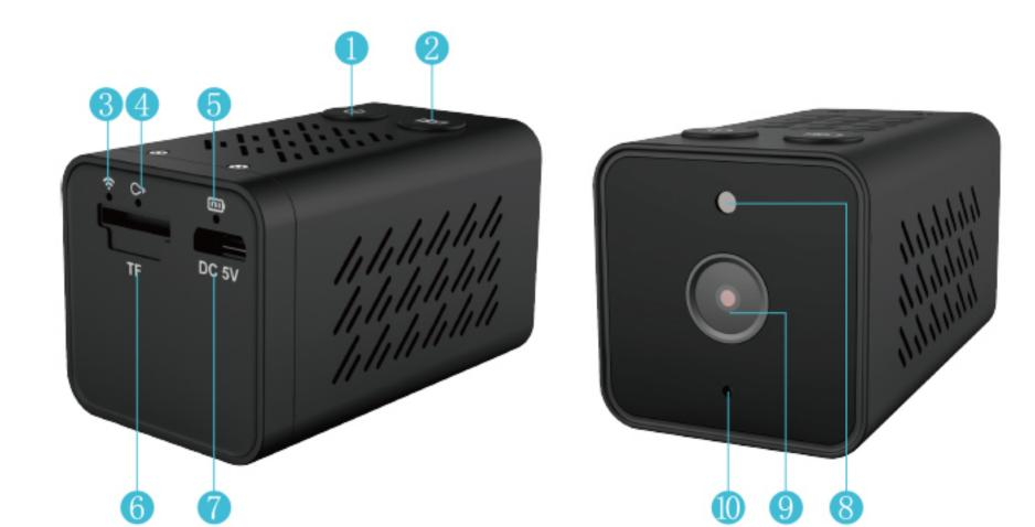
1. Power on/off:press 2s to power on; press 3s to power off. 2. Recording/Reset button: short press to recording, then press again to stop, Press 8s to reset factory setting . 3. Wifi indicator: 3.1 Flashing is AP mode 3.2 Constantly light is internet connected.
