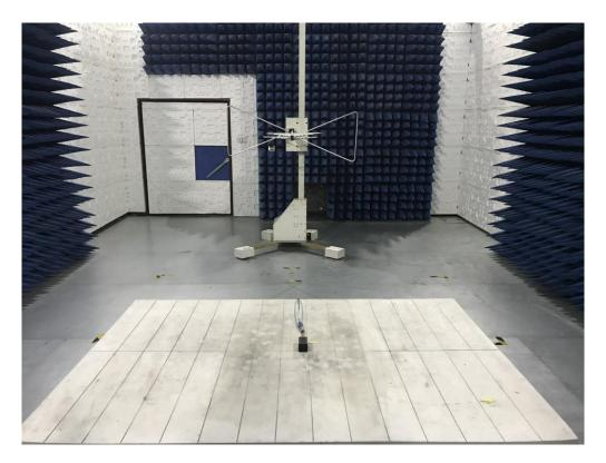
FCC RADIATED EMISSION TEST SETUP ABOVE 1GHZ
