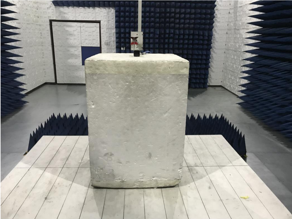
FCC RADIATED EMISSION TEST SETUP ABOVE 1GHZ
