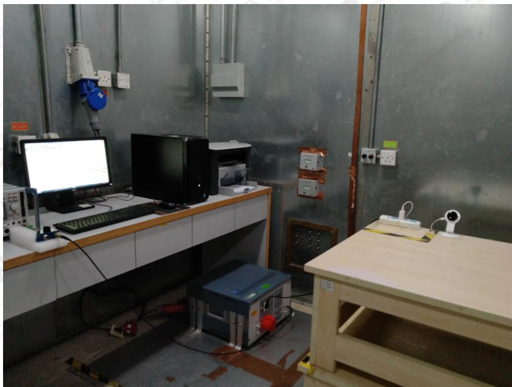
RADIATED EMISSION TEST SETUP
