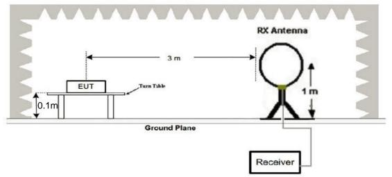
(2) Radiated Emission Test-Up Frequency 30MHz~1GHz
