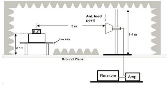
(3) Radiated Emission Test-Up Frequency Above 1GHz
