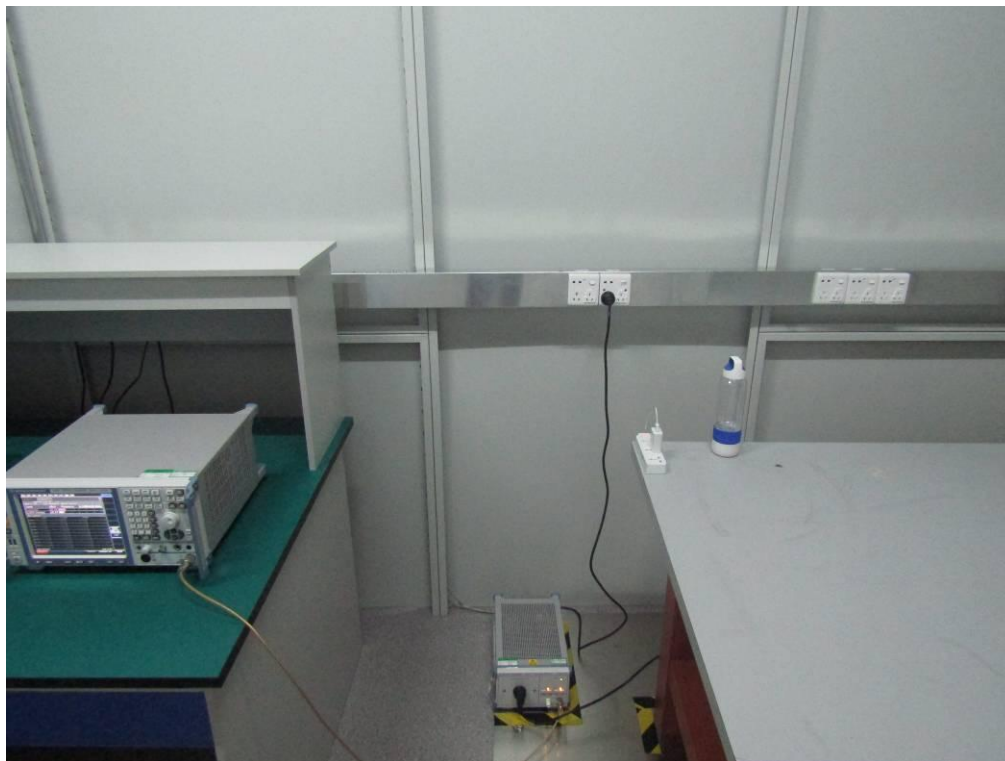
FCC RADIATED EMISSION TEST SETUP
