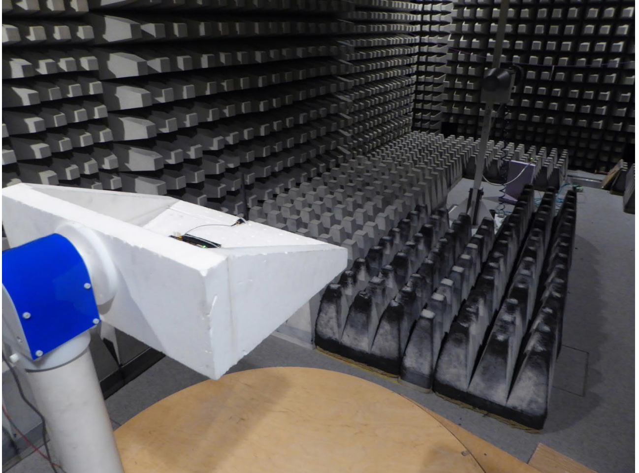
Test setup fully anechoic chamber 1 – 12 GHz
