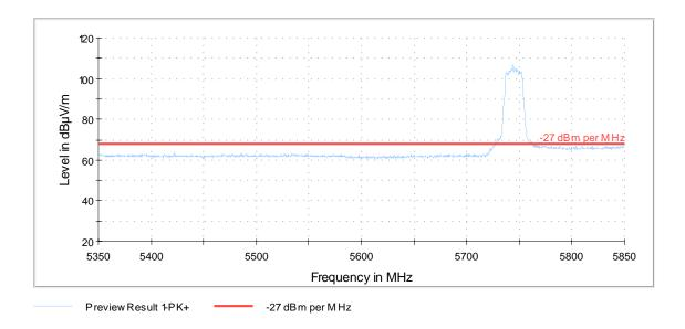
For comparison reasons the limit was converted to a field strength limit line
