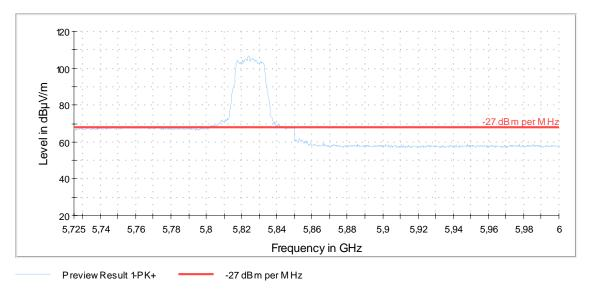
The variation of the peak and average amplitude @ 5.850 GHz is caused by an increased internal attenuation of the measuring receiver to prevent the equipment from overloading.
