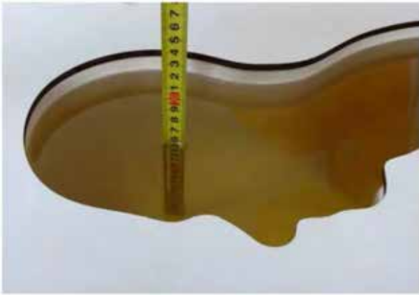
Liquid depth in the head phantom (835MHz)
