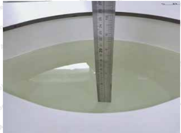
Liquid depth in the body phantom (2450MHz)
