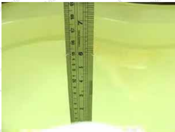
Photo of Liquid Height for Head SAR
