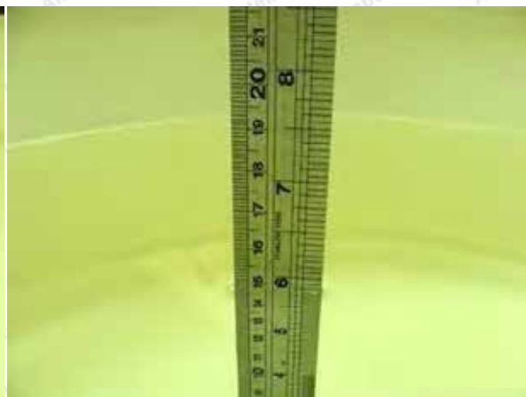
Photo of Liquid Height for Body SAR
