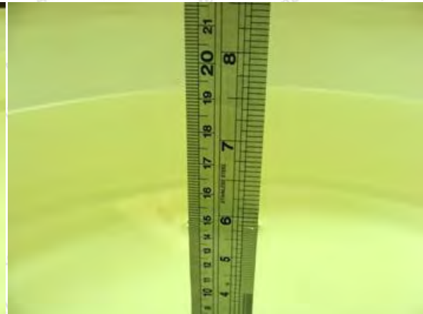
Photo of Liquid Height for Body SAR
