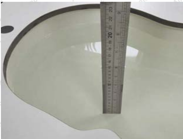
Liquid depth in the head phantom (2450MHz)
