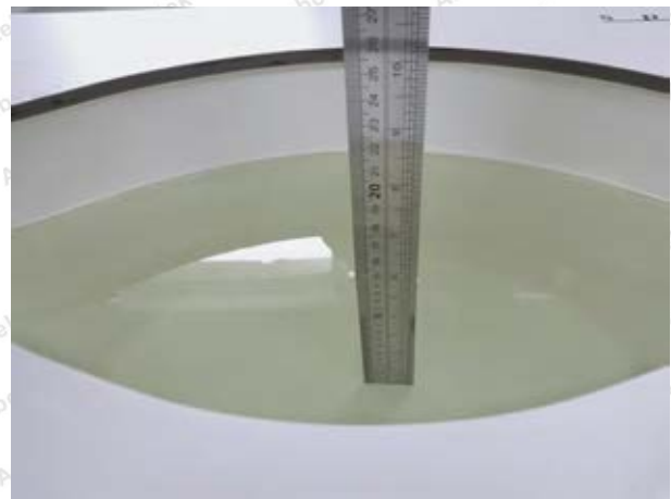
Liquid depth in the body phantom (2450MHz)
