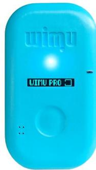
The following symbol will show on the display when the LED light turns red. This means the device is collecting data from the available sensors.
