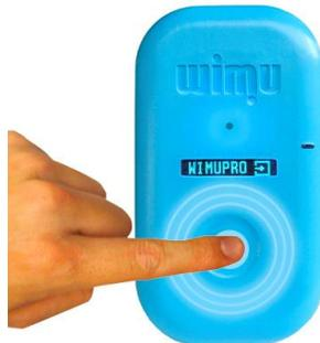
2. **OFF** Press quickly (less than 1 second approx.) the ON/OFF button 4 times in a row. Try it again if the device does not turn off.
