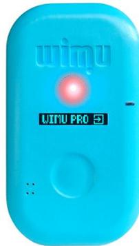
The following symbol will show on the display when the LED light turns green. This means the GPS function of the device is active.
