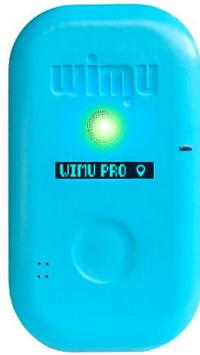
The following symbol will show on the display when the LED light turns green. This means the device is connected to the Heart Rate/GPS/UWB fix monitor device.
