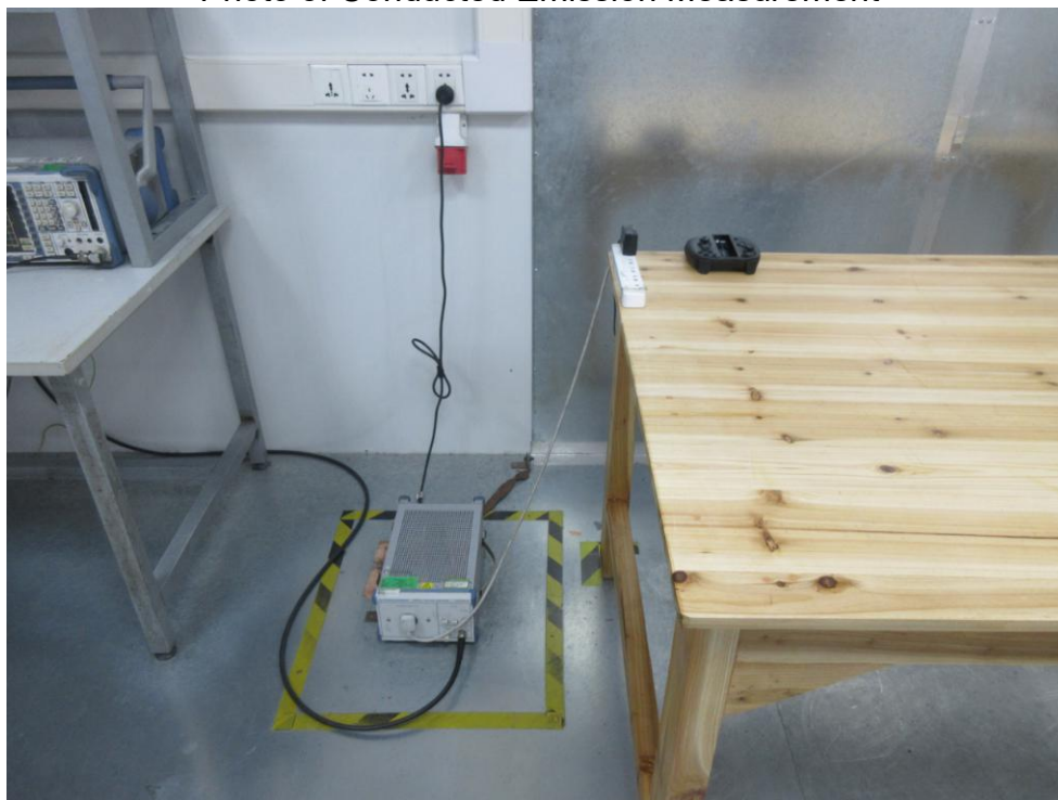
FCC ID:2AQOPIX-SW156 Photo of Conducted Emission Measurement
