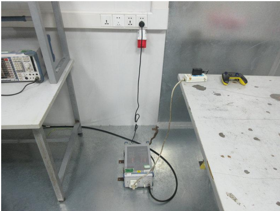
Photo of Conducted Emission Measurement
