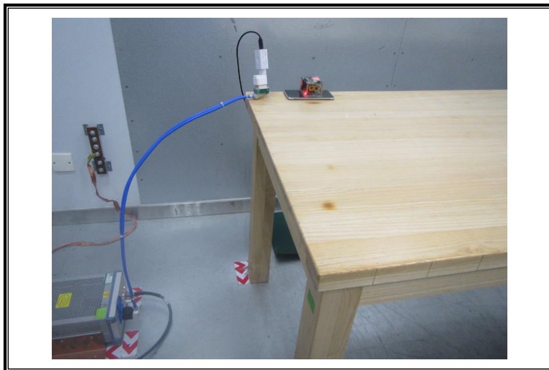
POWERLINE CONDUCTED EMISSIONS MEASUREMENT SETUP
