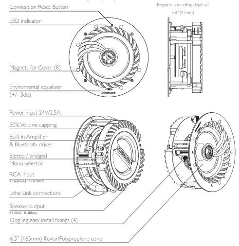
In built over voltage, under voltage, over temperature, and short circuit protection, if there is an electrical fault, the power supply to the amplifier will cut off automatically and restart when the speaker has stabilised.
