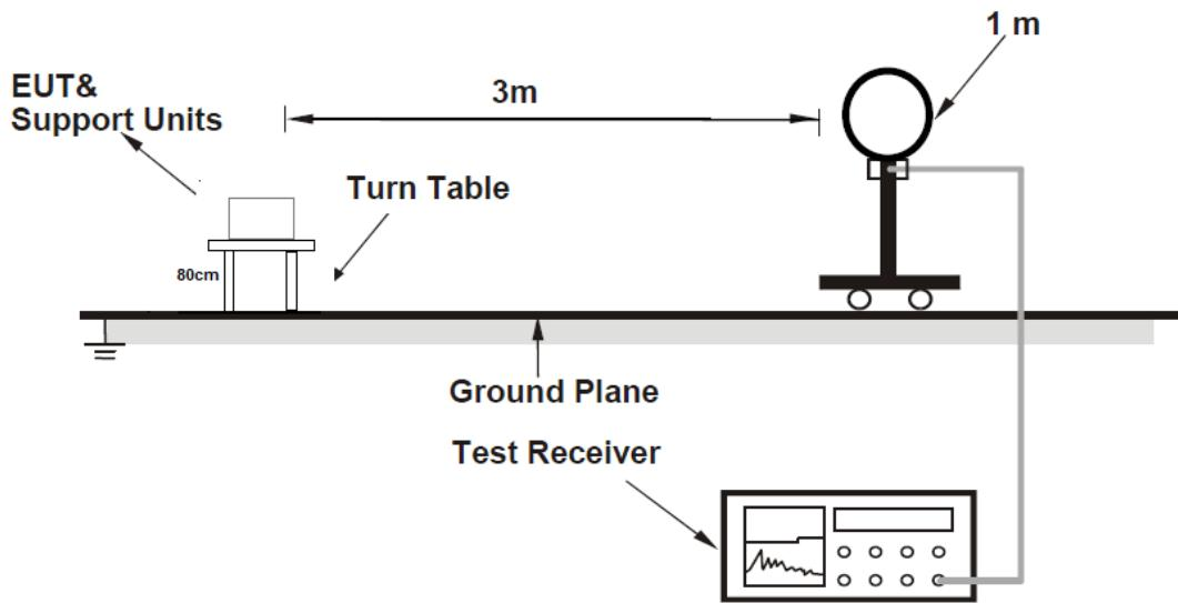
For Radiated emission between 30MHz~1000MHz
