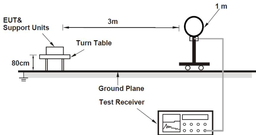
For Radiated emission 30MHz to 1GHz
