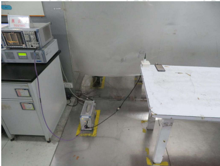
Conducted Emissions Test Setup
