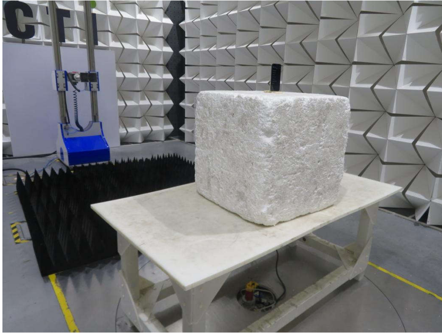
Radiated spurious emission Test Setup-3(Above 1GHz)
