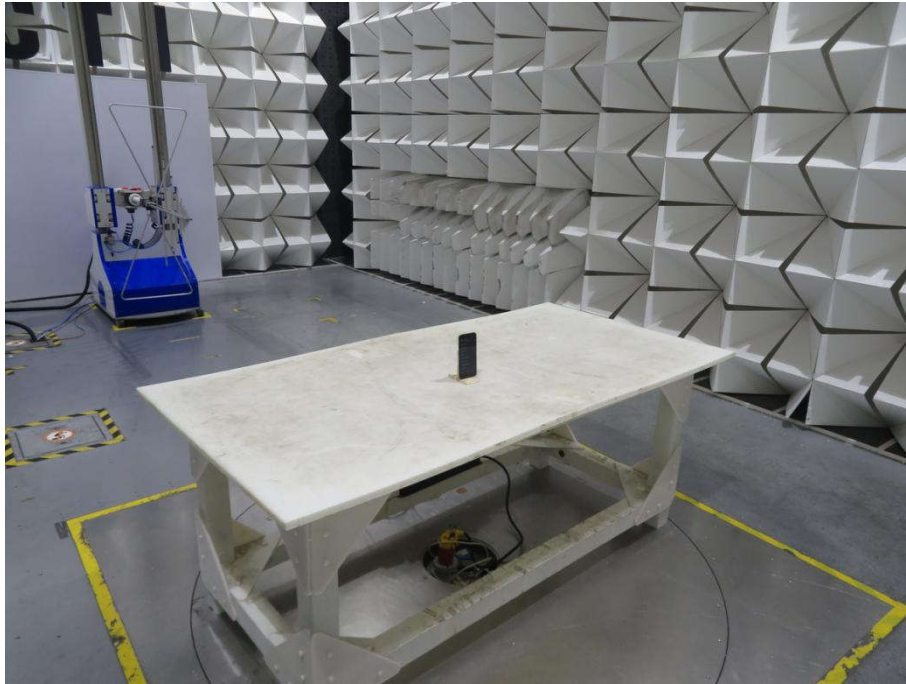
Radiated spurious emission Test Setup-1(Below 1GHz)
