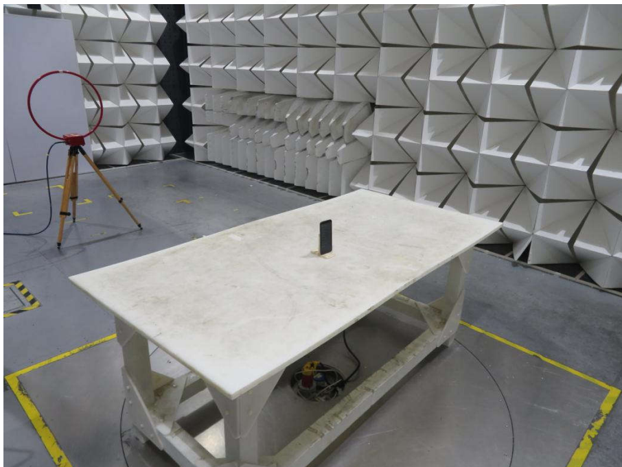
Radiated spurious emission Test Setup-2(Below 30M)
