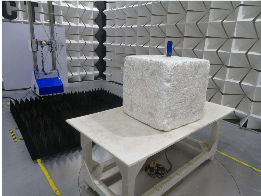
Radiated spurious emission Test Setup-1(Below 1GHz)
