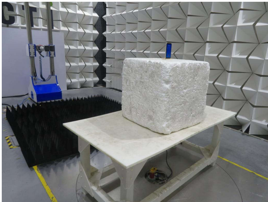
Radiated spurious emission Test Setup-2(Above 1GHz)
