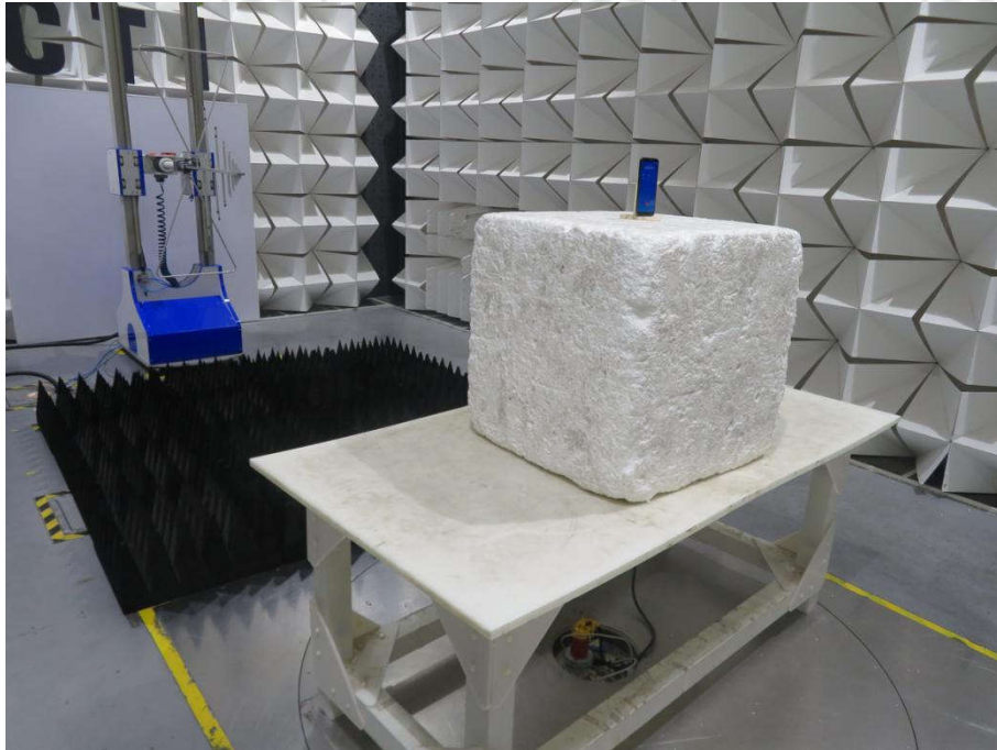
Radiated spurious emission Test Setup-1(Below 1GHz)
