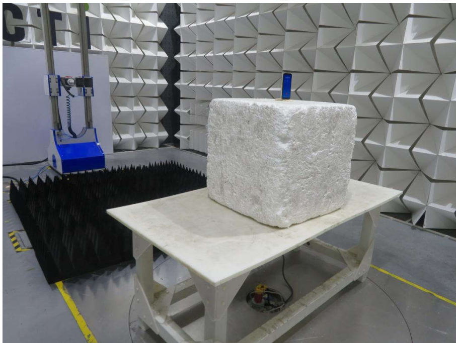
Radiated spurious emission Test Setup-2(Above 1GHz)
