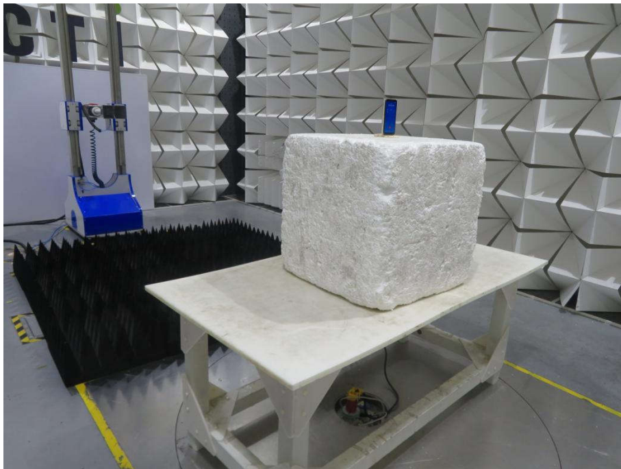
Radiated spurious emission Test Setup-2(Above 1GHz)
