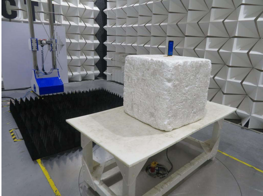
Radiated spurious emission Test Setup-1(Below 1GHz)
