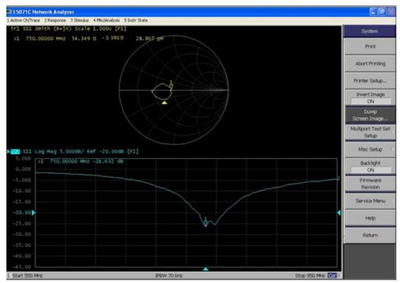
D750V2, serial No. 1103 Extended Dipole Calibrations
