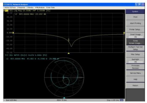
D835V2, serial No. 4d141 Extended Dipole Calibrations
