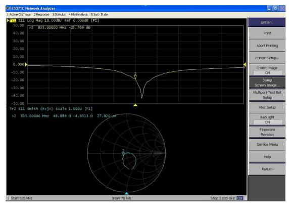
D835V2, serial No. 4d141 Extended Dipole Calibrations
