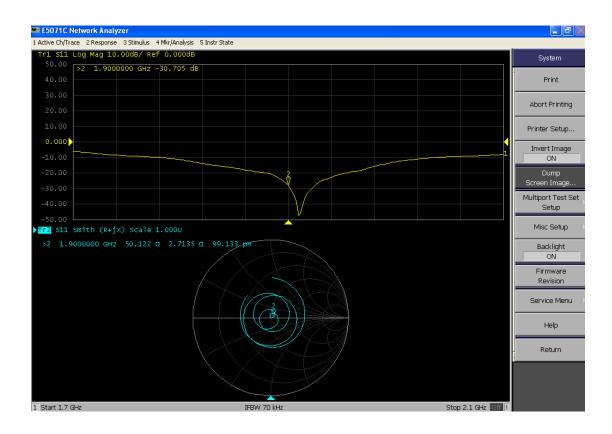
D1900V2, serial No. 5d162 Extended Dipole Calibrations
