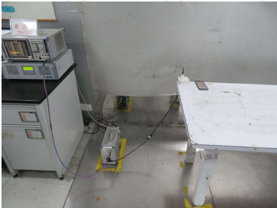
Conducted Emissions Test Setup
