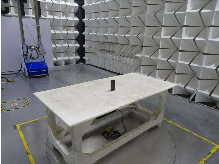
Radiated spurious emission Test Setup-1(Below 1GHz)
