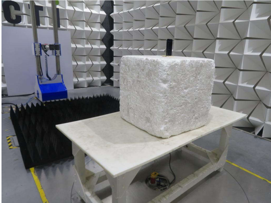
Radiated spurious emission Test Setup-3(Above 1GHz)
