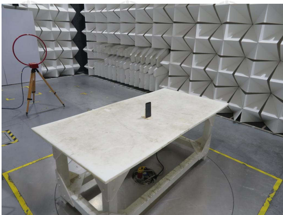
Radiated spurious emission Test Setup-2(Below 30M)
