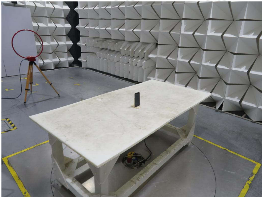
Radiated spurious emission Test Setup-2(Below 30M)
