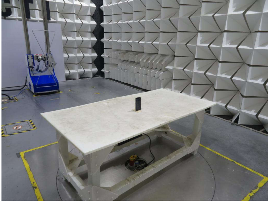
Radiated spurious emission Test Setup-1(Below 1GHz)
