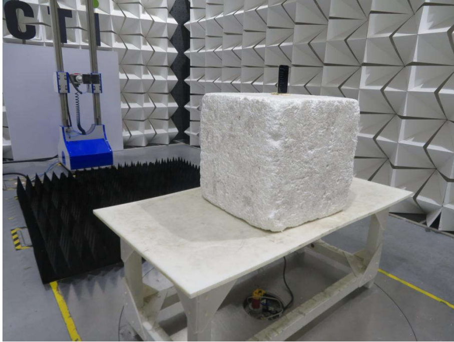
Radiated spurious emission Test Setup-3(Above 1GHz)
