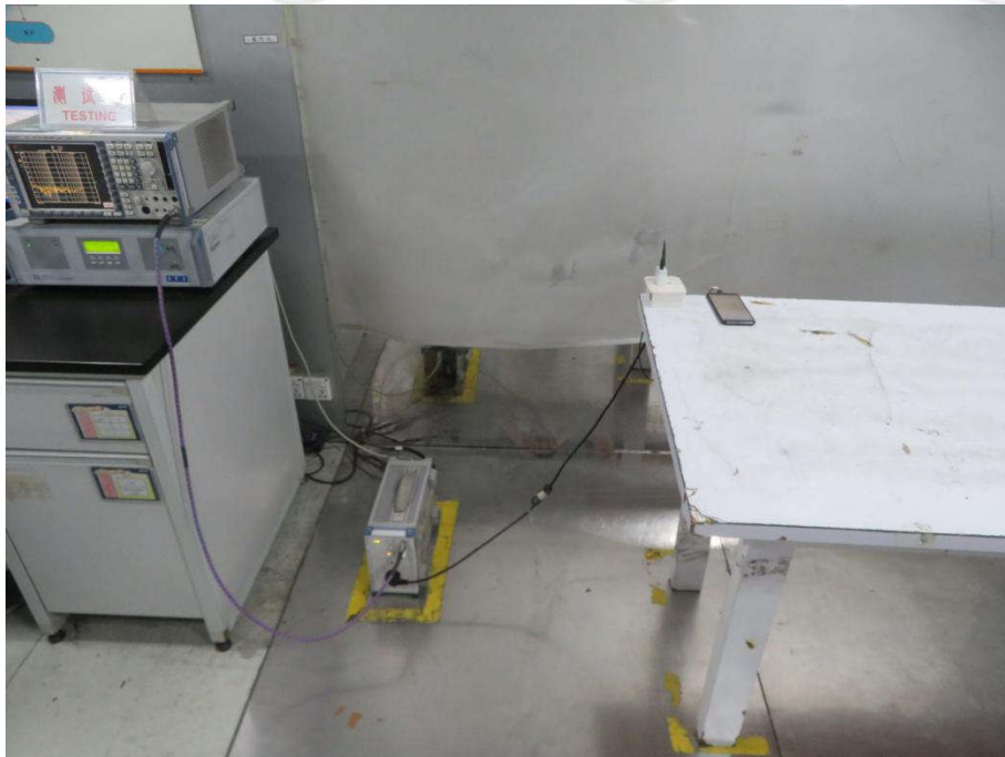
Conducted Emissions Test Setup
