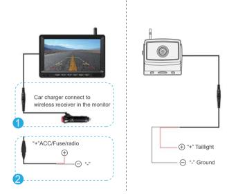
Note: Of connecting power directly to battery, the cameras always ON and therefore candrain battery. Therefore it is recommended to connect power to an ignition switched accessory power source.
