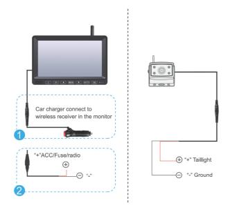
Note: Of connecting power directly to battery, the cameras always ON and therefore candrain battery. Therefore it is recommended to connect power to an ignition switched accessory power source.
