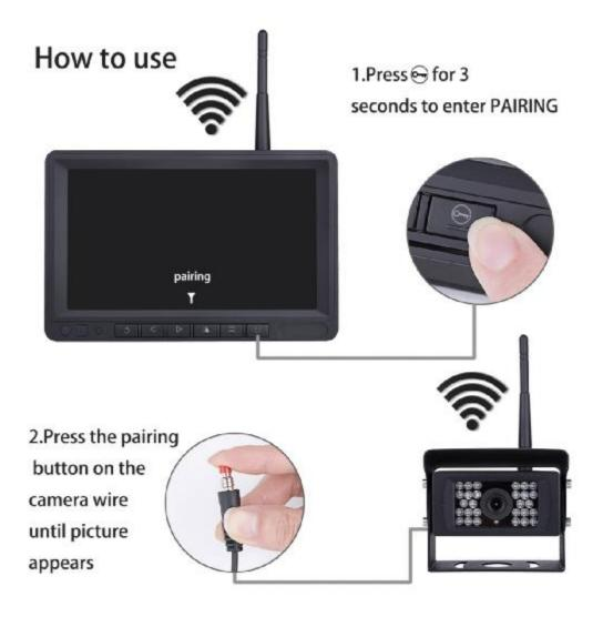
Note: the system has been paired successfully at the factory, and if you need to rematch, refer to steps 1 and 2 above. Please make sure the camera is receiving power when you pair.
