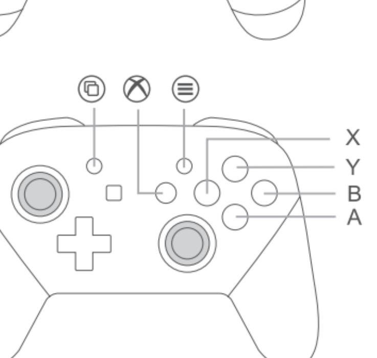
Pairing button, Holding 2 seconds to have scrolling Led for pairing.
