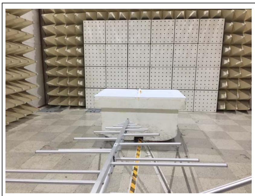
**3. Photo of Radiated Spurious Emission Test (Above 1 GHz)**
