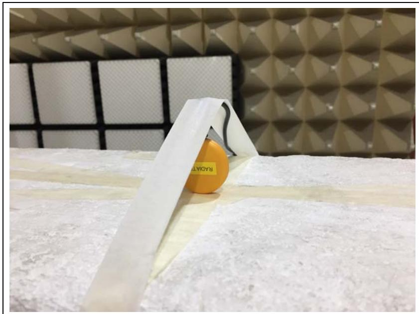
**2. Photo of Radiated Spurious Emission Test (Below 1 GHz)**
