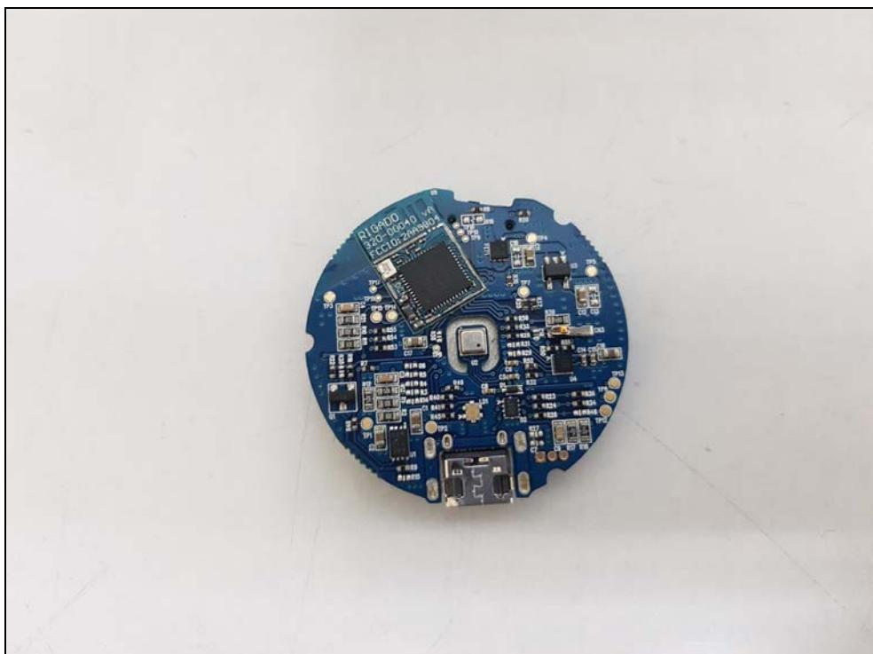
**View of Bluetooth module (with Shielding)**
