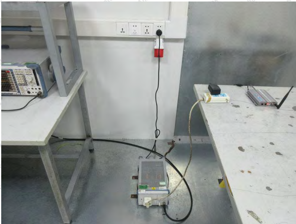
Photo of Conducted Emission Measurement
