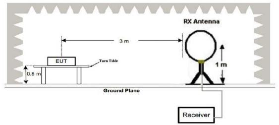
(2) Radiated Emission Test-Up Frequency 30MHz~1GHz
