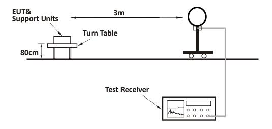
For Radiated emission 30MHz to 1GHz:
