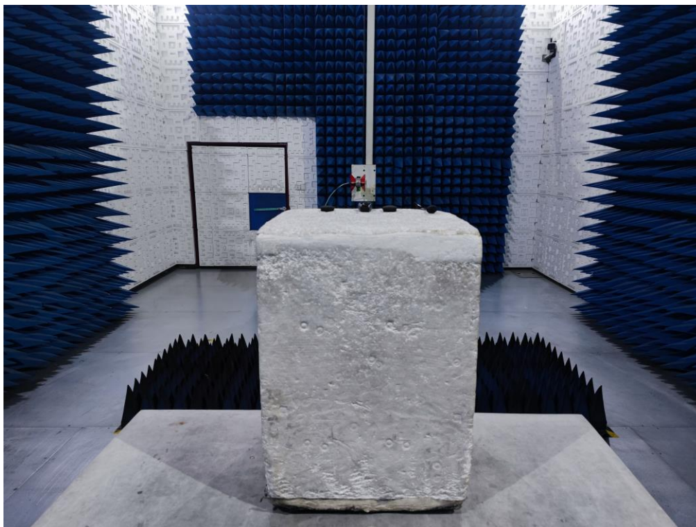
RADIATED EMISSION TEST SETUP ABOVE 1GHz
