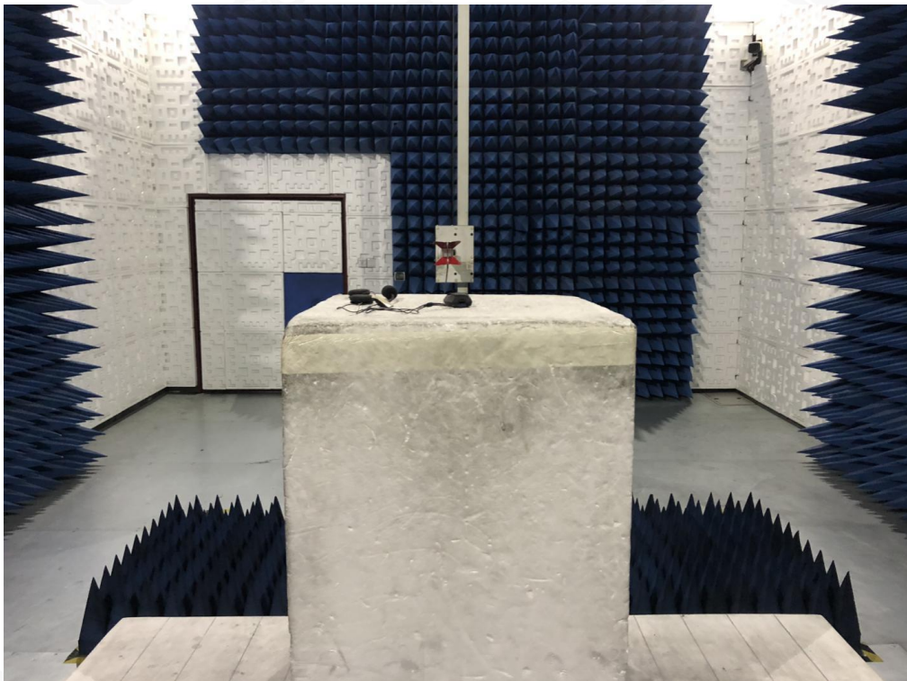
RADIATED EMISSION TEST SETUP ABOVE 1GHZ
