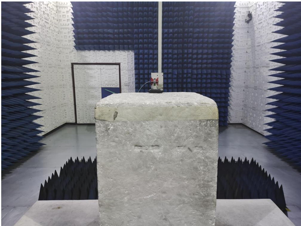
RADIATED EMISSION TEST SETUP ABOVE 1GHZ
