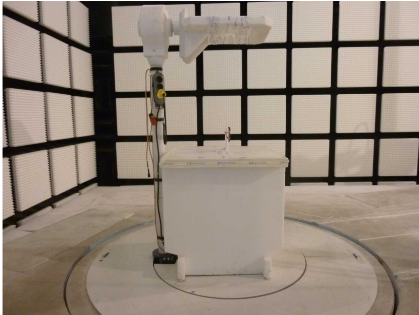
Photo 7: MYUB-PLUG at the anechoic chamber, loop antenna test setup
