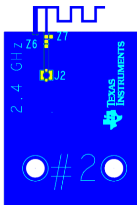
Figure 14. Board #2 – Compact 2.4 GHz PCB Antenna
