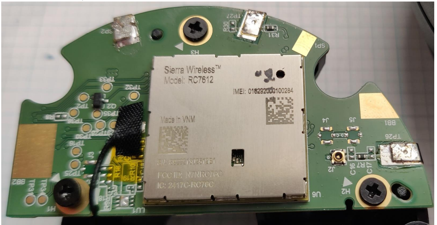
03 - LTE board close-up, front
