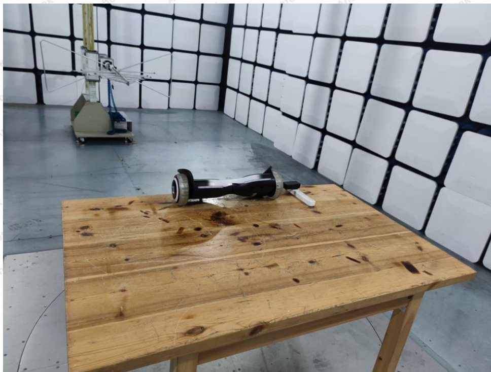
Photo of Radiation Emission Test
