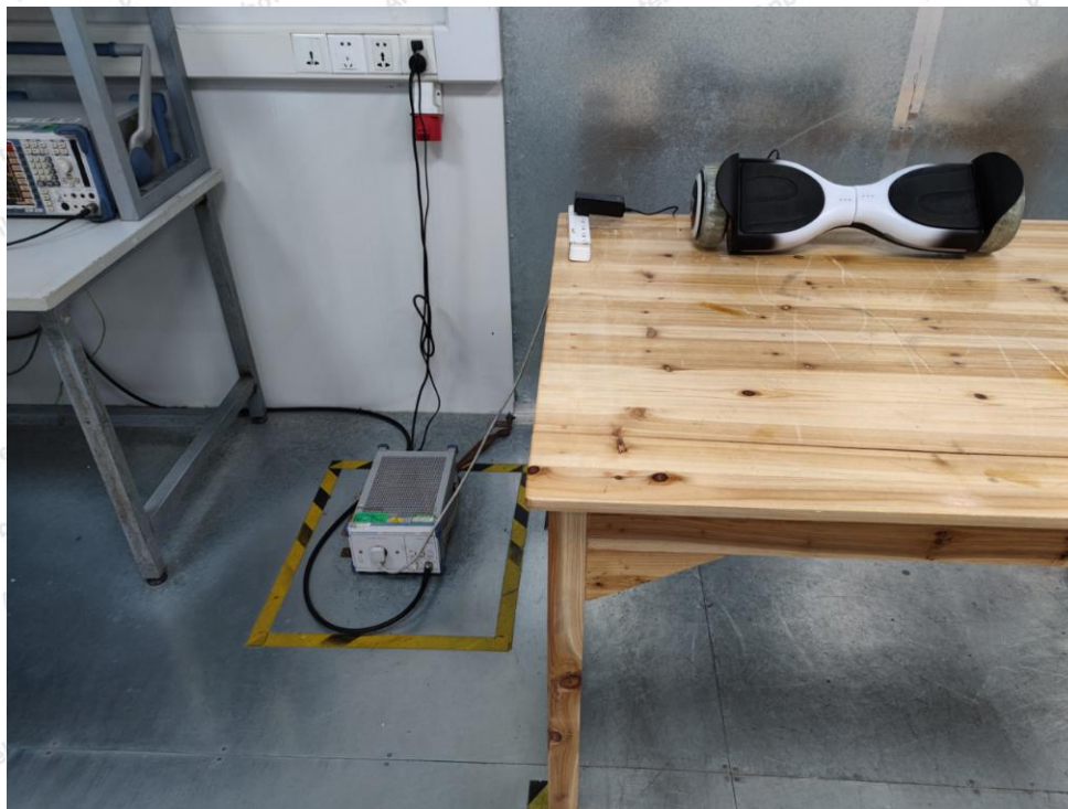
Photo of Conducted Emission Measurement
