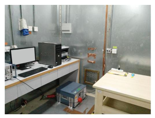
RADIATED EMISSION TEST SETUP
