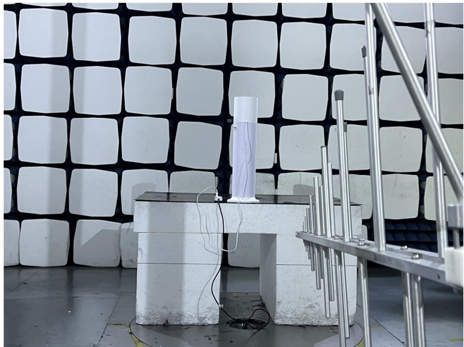
Radiation Emission Test Setup (30MHz to 1GHz)
