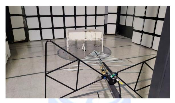
HINGE HEALTH, INC. HINGE SENSOR MODEL: H4 FCC SUBPART B AND C; RSS-210 AND RSS-GEN RADIATED EMISSIONS – AC MODE – BELOW 1 GHz
