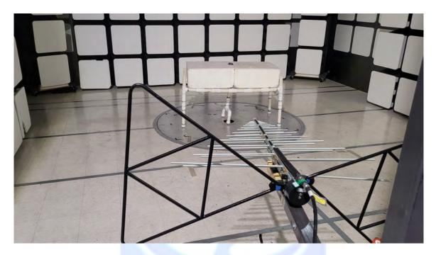
HINGE HEALTH, INC. HINGE SENSOR MODEL: H4 FCC SUBPART B AND C; RSS-210 AND RSS-GEN RADIATED EMISSIONS – BATTERY MODE – BELOW 1 GHz
