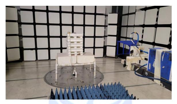
HINGE HEALTH, INC. HINGE SENSOR MODEL: H4 FCC SUBPART B AND C; RSS-210 AND RSS-GEN RADIATED EMISSIONS – AC MODE – ABOVE 1 GHz
