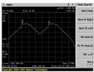
(1Mbps) Channel Separation plot on channel 39-40
