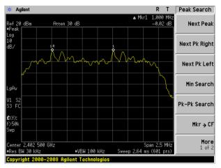
(2Mbps) Channel Separation plot on channel 39-40
