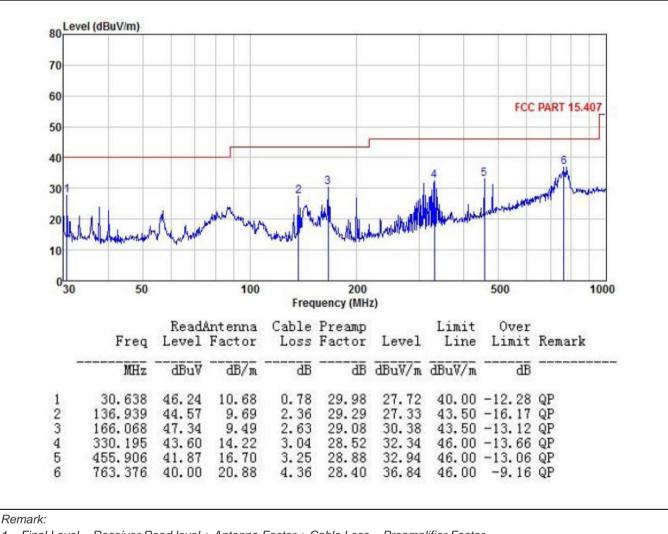
1. Final Level = Receiver Read level + Antenna Factor + Cable Loss – Preamplifier Factor.
