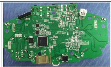
The antenna is PCB antenna. The best case gain of the antenna is 0.31dBi.
