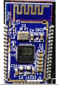
The antenna is PCB antenna. The best case gain of the antenna is 0dBi.
